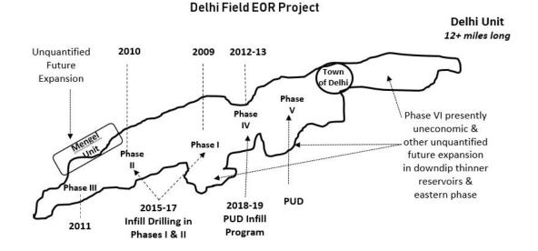
After the May 2006 conveyance, Denbury as the operator originally planned six primary phases for the installation of the  $CO_2$  flood in the Delhi field. Four of these six phases have been completed as of June 30, 2021, and two remain undeveloped. One of the remaining two phases (Phase V) is reflected as proved undeveloped in our current reserves report and the other (Phase VI) was removed from proved reserves as it was not deemed economic due to distant location and oil price.
